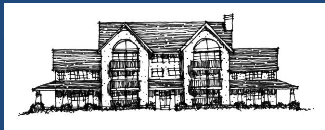
Taller Buildings should be stepped back in height with lowest toward the street or adjacent single-family homes
