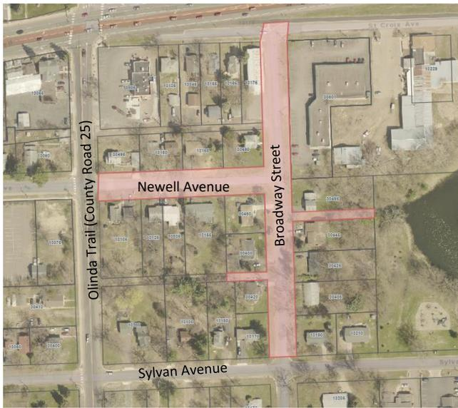
**What's Been Going On?** Over the past couple months, private utility contractors, specifically Xcel and Midco, have been upgrading and relocating private utilities within the project area in advance of the street improvements. New gas main was installed on both sides of the street and the existing fiberoptic lines were relocated to avoid conflict with the new utilities.
